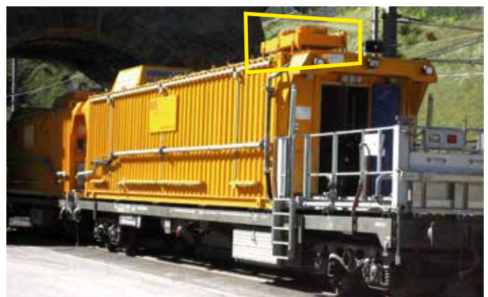
Radiator mounted separately on wagon roof
