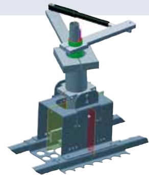
eMove Motor Mounting with Rudder Control
