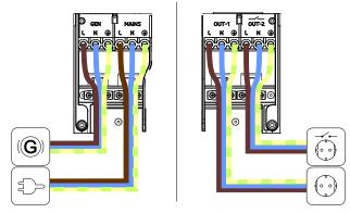
Figure 5-1: AC terminal connections
