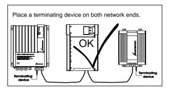
Connections between the devices are made by standard straight UTP patch cables.
