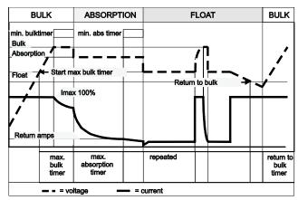
Figure 3-2: 3-Step+ charge system
