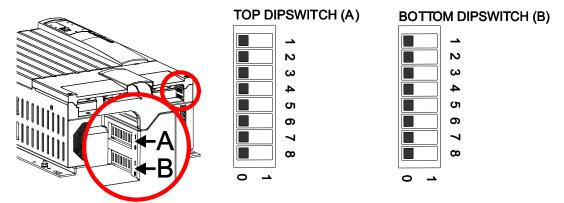
Figure 6-1: DIP-switches and cover print
