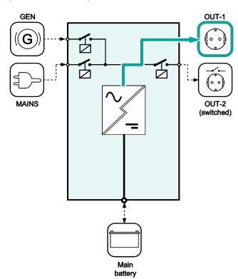
Figure 3-3: Inverting mode
