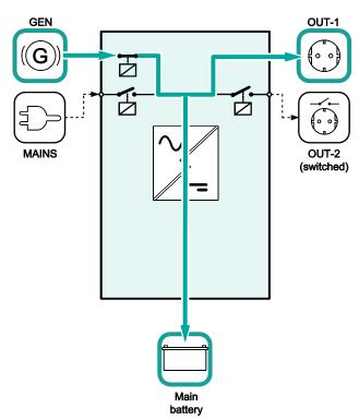
Figure 3-4: AC power from Generator input
