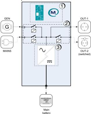
Figure 3-1: Working principle of the Mass Combi Pro
