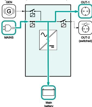
Figure 3-5: AC power from Mains input
