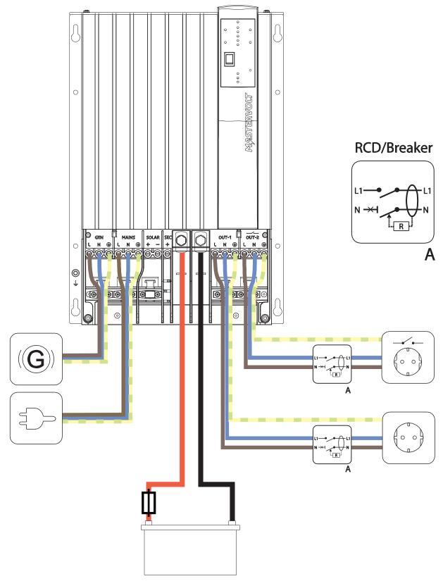
Figure 5-4: Installation overview for one Mass Combi (stand-alone operation)
