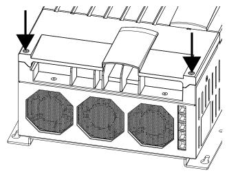
Figure 5-2: Removal of the front lid
