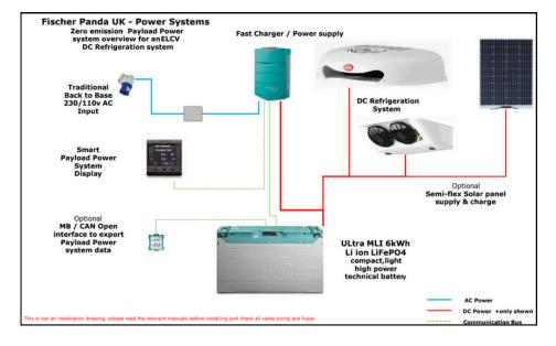
The teams from GAH, Mertrux, and Fischer Panda UK | Power Solutions combined forces and delivered a fully integrated zero emission solution. Engineers and specialists from different fields. such as refrigeration, transportation, installation and power, came together to design and implement the system, as well as train all operators in efficient use and aftersales support. project was carefully thought through over six months, with the first vehicle commissioned at the end of March 2025.
