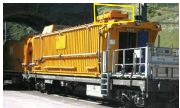
Radiator mounted separately on wagon roof
