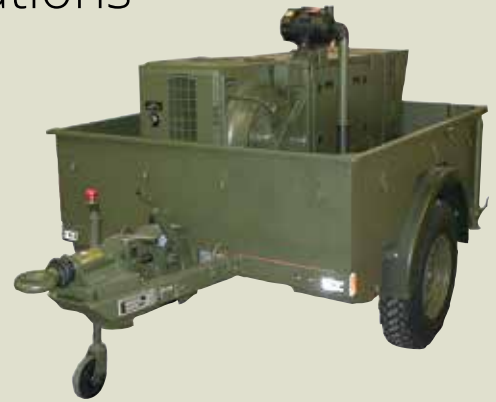
Complete unit, cooling, fuel, 6 kW generator and electrical systems all mounted on frame. Vertical mounted radiator is rotated 90°, for cooling efficiency in high side trailer.
