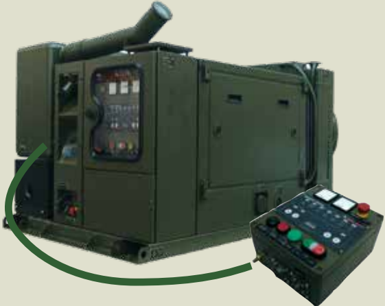
Complete unit, cooling, fuel for 72 hours, 15 kW generator and electrical cabinet mounted on frame. Major electrical functions via remote control unit.
