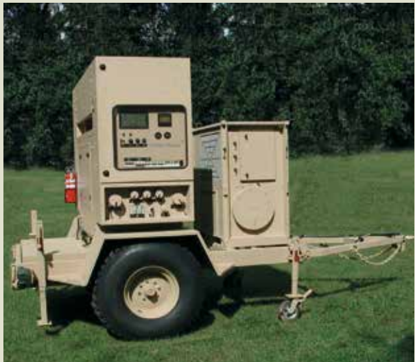
Teamwork:Trailer Mounted 40kW Generator with Fischer Panda's own ECU 6000 providing 75.000 BTU specifically designed for military applications.
