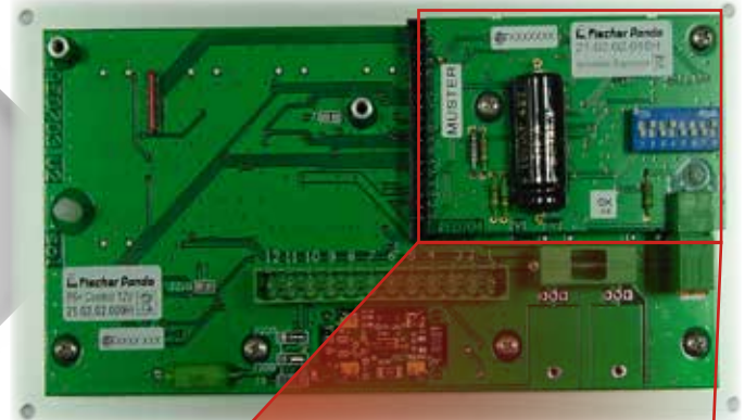
Automatic system add-on connected to rear of P6+ Panel
